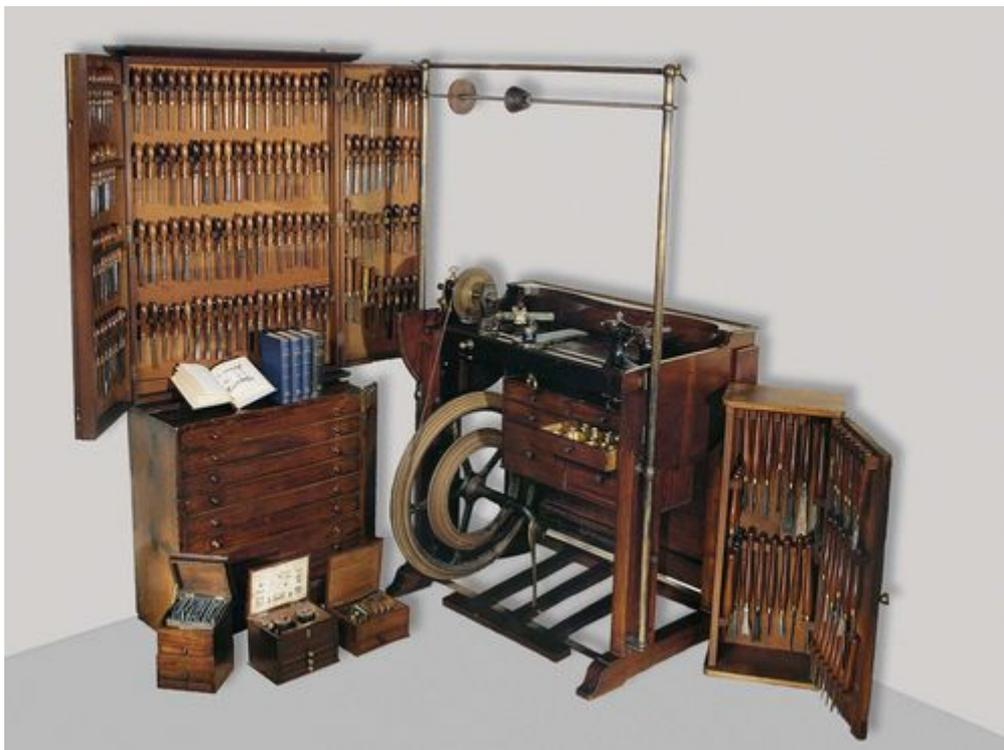
**A RARE TURNING LATHE WITH A NUMEROUS TOOLS IN 2 LARGE AND 3 SMALL BOXES, by the company Holzappfel, London, 1824. Mahogany, cast iron, brass and steel. Pedal driven.**
